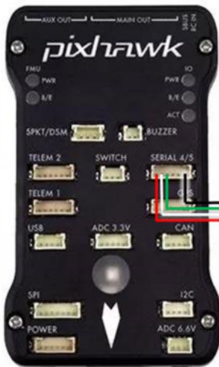
Figure 2 Schematic Diagram of Connecting TF02 with SERIAL4/5 Interface (Serial Port 4/5) of Pixhawk
