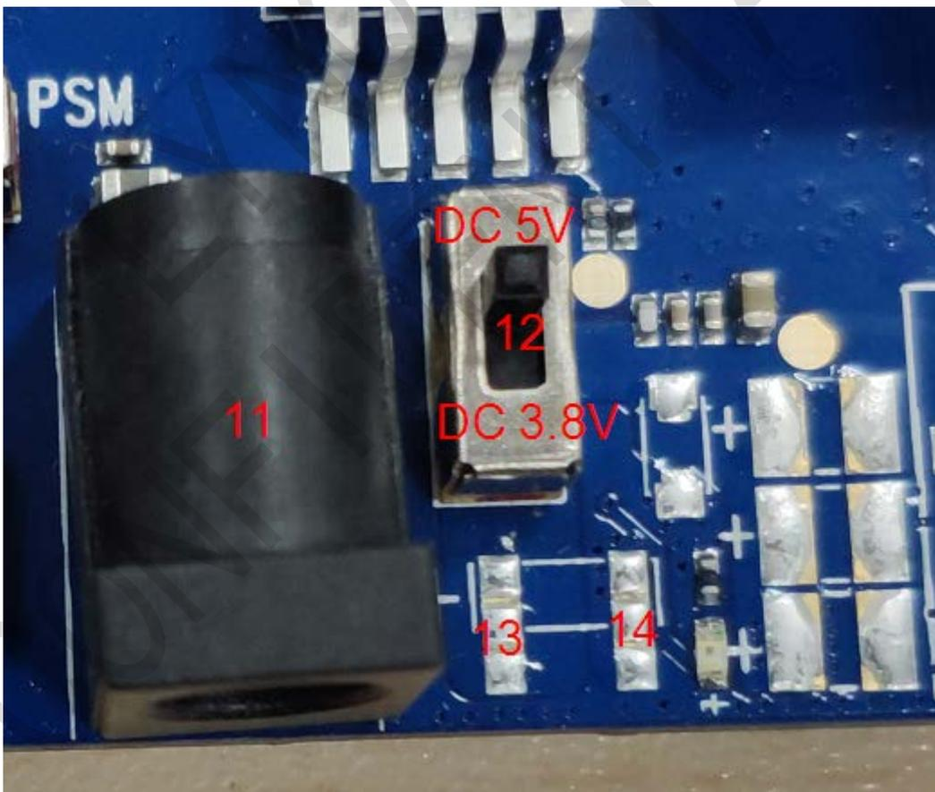
Figure 2-1 L651\_EVB DC Power interface and Power Switch
