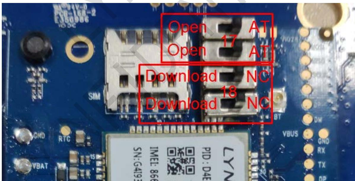
Figure 2-7 Serial port switch
