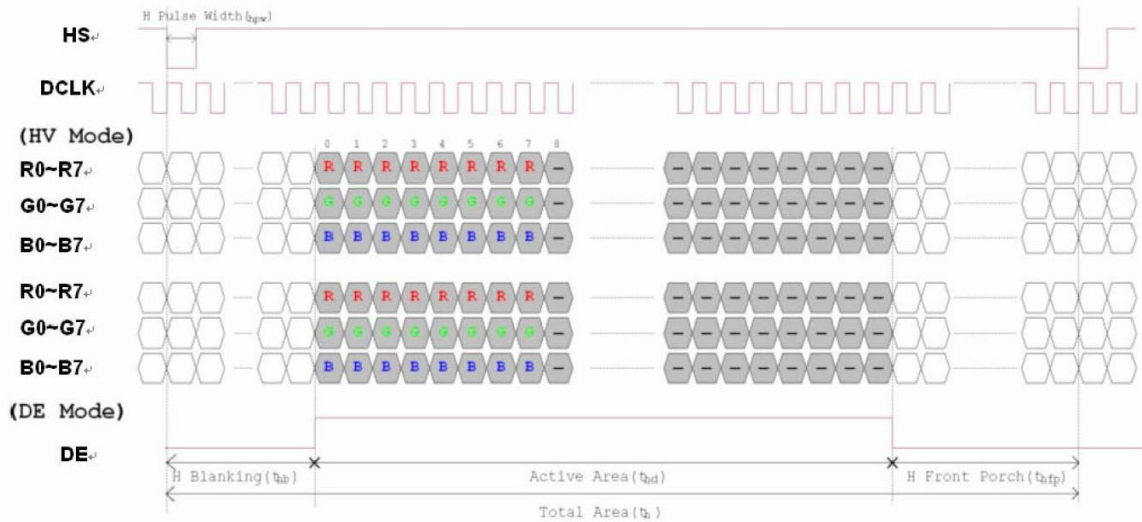
Figure 7. Horizontal input timing diagram
